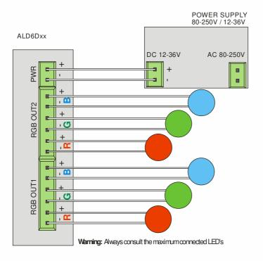
Always calculate the appropriate power supply depending on the LED fixture used. If you need help, contact the manufacturer at sales@srs-group.com. By doing so you will avoid lots of problems and burned fixtures!!!
