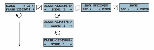
The flash scene is a scene mode, where scenes are called by a single press of button. When any other button on HLC is pressed, the other scene is called. You can preset up to 8 scenes. A scene that is to be Flash must be added to the Flash scene list. Turn the Encoder until you get to the desired scene number and confirm by ENTER button. To remove a scene from the Flash scene list, turn the Encoder to the scene number and press the ESC button. A single press of the Encoder saves all settings.
