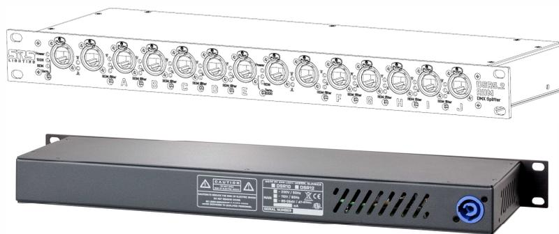
The DSR5.2-RDM-N is a 19" 1U rack-mount double-group 5-channel splitter / booster of both the DMX and RDM signal. Every output features LED indication of the DMX/RDM status and an RDM filter, and is optically isolated up to 1000V. The unit also provides a true output for easy daisy-chaining of other DMX/RDM devices.
