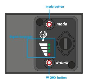
For the DMX operation, turn off the W-DMX module by holding the MODE button until both W-DMX and MODE buttons light in red color.
