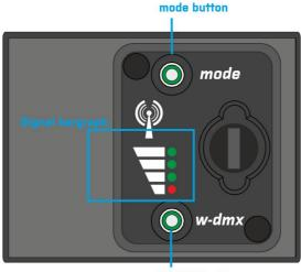
For the W-DMX operation, turn on the W-DMX module by holding the MODE button until it lights in green color.
