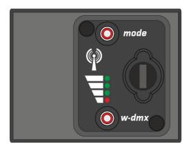
2. W-DMX is ready to be linked. DST4W works as a receiver of the W-DMX signal without a link to the transmitter.
