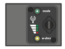
4. W-DMX is linked to the Transmitter and is receiving the DMX signal. Both indicators are in green color. Bargraph is working and showing the W-DMX signal strength.
