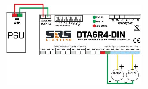
By default, the first 4 DMX channels are RELAY 1-4 and then another 6 DMX channels are analog outputs 0/+10V. Switching relay from 0 to 100% is performed by the value of 25 on the DMX channel according to the DMX start address setting. Without power, the CMNx and NCx contacts are closed
