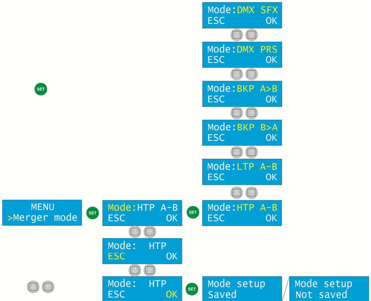
Press "SET" to enter the *Merger mode*. Press "SET" again to adjust the merger mode. Use the arrow keys to reach the desired option and confirm by "SET". Scroll down to "OK" and press "SET" to save the settings.
