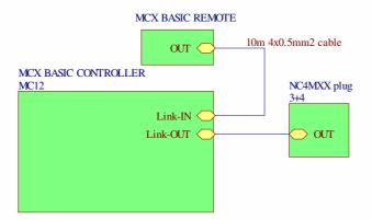
During operation, the NC4MXX plug must be connected to the last controller in chain
