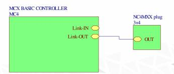
During operation, the NC4MXX plug must be connected to the last controller in chain
