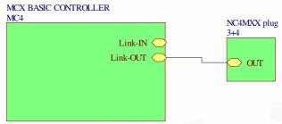
During operation, the NC4MXX plug must be connected to the last controller in chain
