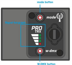
For the DMX operation, turn off the W-DMX module by holding the MODE button. The MODE button should be RED.
