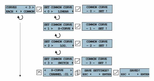
Press the left button to select the curves for each channel individually or the right button to set one common set of curves for all channels.
