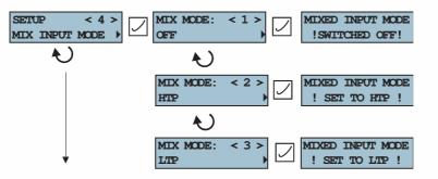
The dimmer is switched to the HTP or LTP mix mode now. In this mode, the dimmer is controlled via DMX and 0-10V input at same time.
