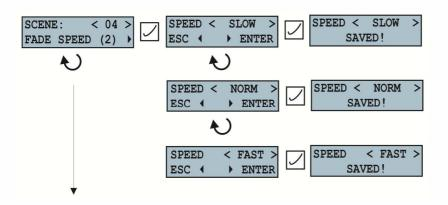
The fade speed can be set in three timeframes: SLOW, NORMAL or FAST. According to the setup, the scene will be changed to the selected speed when the scene is called.
