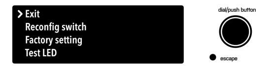
Rotate the data button to move the cursor to the desired option. Press the data button to confirm your choice. The VLAN-toolbox will then perform the selected action.
