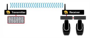
• Point to multipoint operation: In this mode, one W-DMX transmitter (W-DMX TX) is communicating with up to 48 W-DMX receivers (W-DMX RX).
